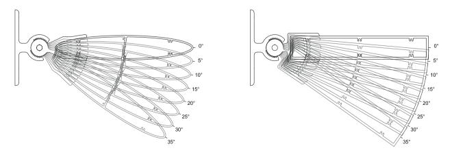
Blade angle can be customized by using the internal bracket grooves
